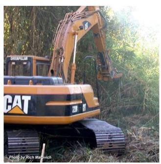
Equipment used to remove arundo along Pleasants Creek and Putah Creek. Arundo is ground to mulch and dried in place. The mulched stems can suppress weeds and reduce erosion in the transition period in which native plants are restored.
