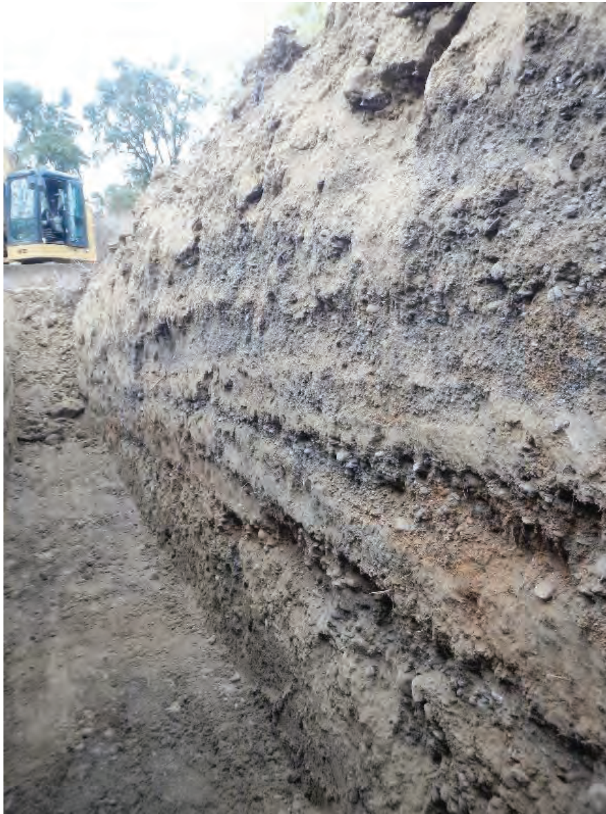
Figure 2. Trench in Winters. Sorted and stratified sedimentary layers.
